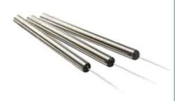
The FC Series fiber optic coupler is based on Agiltron's fused biconical taper technology and compact packaging structure. It features good uniformity, low excess loss and very low polarization sensitivity. The device is ideal for splitting or combining light with exceptional performance over a wide wavelength range.
